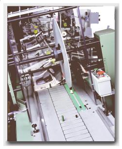
Vacuum drawn through the KR600's flighted chain system keeps the jacket under control, even at higher line speeds.
