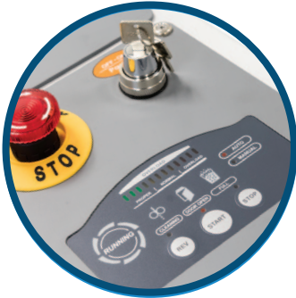
User-Friendly Control Panel: Door Open Sensor, Reverse, Waste Bin Full Indicator
