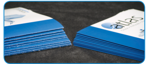
Uncreased folded digital prints (left) are cracked and give the appearance of poor quality. Creased prints (right) have no cracking and look polished and professional.
