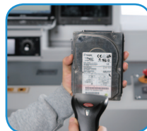
Barcode reader documents hard drives being shredded
