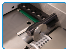
Bottom-suction air feed system
